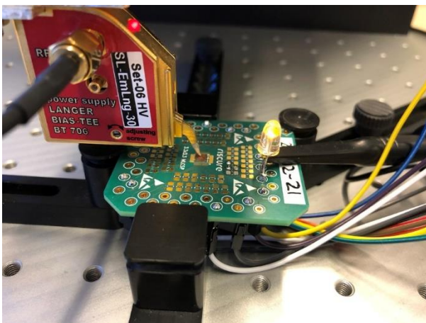
Figure 25 Langer probe positioned on the spot with the best signal
