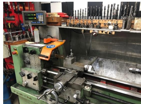
Figure 8 Lathe with PMMA rod inserted
